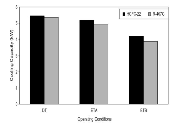
Cooling capacity of HCFC-22 and R407C
